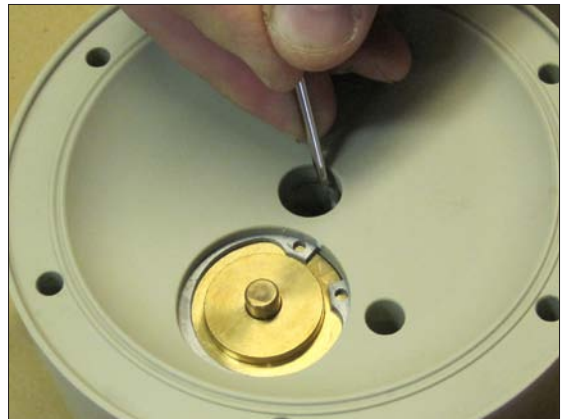
Fig 10. If the shaft sealings (36) seem to be worn out (by internal leakage of air), carefully remove them with a pointed tool. During this operation, the sealing (36) and backup o-ring (47) usually get destroyed, so make sure to have replacement spares available.
