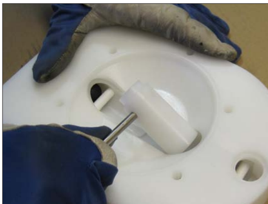
Fig 4. Carefully pull out the the spacer sleeve (19). Please note that force never shall be used for dismantling.
