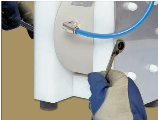
Fig 24. Fasten the nuts (37) alternatingly, with or without washers depending on how much of the thread comes out. If some of the nuts were fastened without washer, unscrew those and put washers underneath. Tighten the nuts according to recommended tightening torques in chapter 5.
