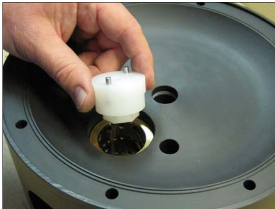
Fig 15. To push out the cylinder, use the other side of the mounting tool that fit into the cylinder.
