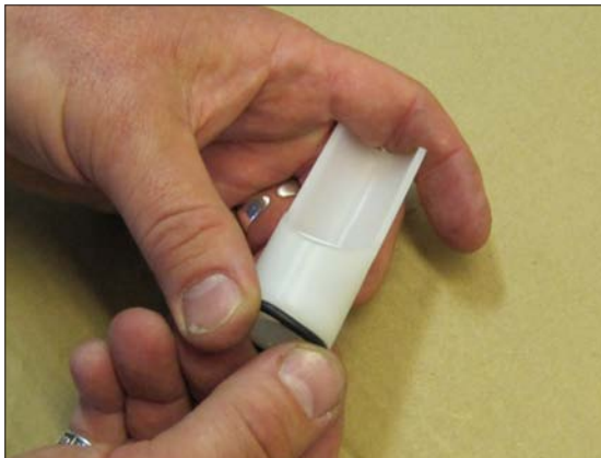
Fig 13. Place the valve ball (23) in the lower valve seat (21) and mount the ball stop (22). Mount the valve seat o-ring (43) at the bottom of the seat (21)
