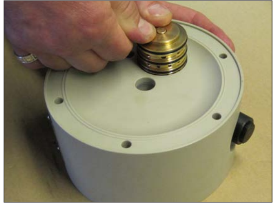
Fig 2. Put a little water on the o-rings (30), other lubricants should not be used. Carefully push the air valve (61) into the housing. Mount the circlip (27) on the remaining side (see fig. 1).
