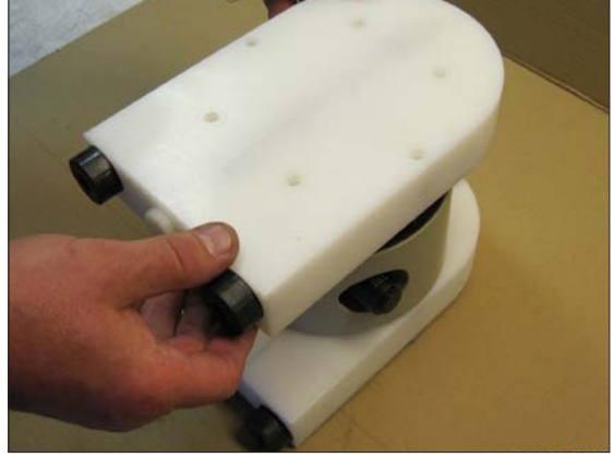
Fig 23. Carefully lift on the remaining housing and the stainless steel side plate with booster.
