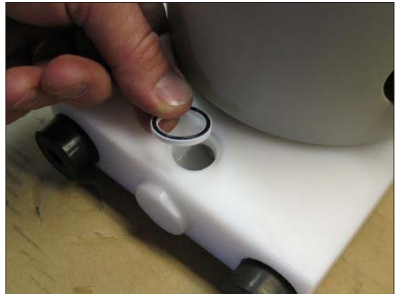
Fig 21. Put the small o-ring (pos 18) in the seat of the housing. On pumps with PTFE diaphragms the PTFE u-ring with its o-ring shall be mounted with o-ring facing upwards (see Fig. 21).
