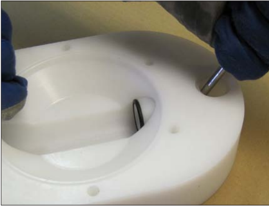
Fig 6. Push out the upper valve seat (20), be careful not to damage the edge of the connection hole.
