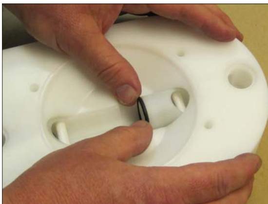
Fig 15. Mount the upper seat assembly; upper seat (20), valve ball (23), ball stop (22) and o-ring (43).
