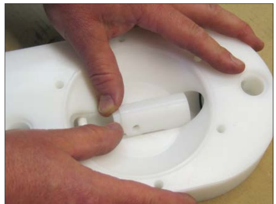
Fig 16. Place the spacer sleeve (19) upside down and press it up towards the the upper valve seat (20).
