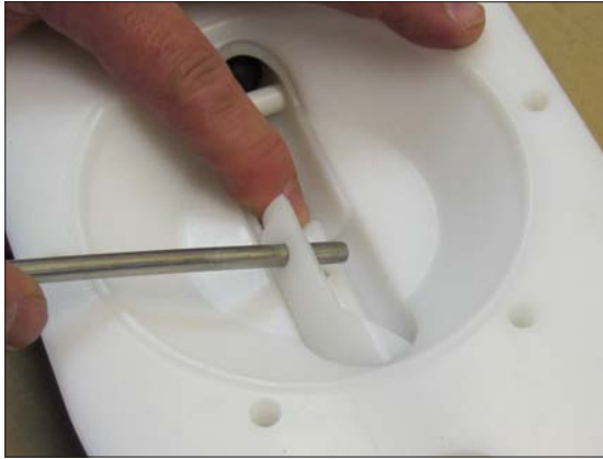
Fig 17. Put one of the pin screws into the hole of the spacer sleeve (19) and turn it gently. Knock also carefully with a plastic hammer to easier force down the spacer sleeve.
