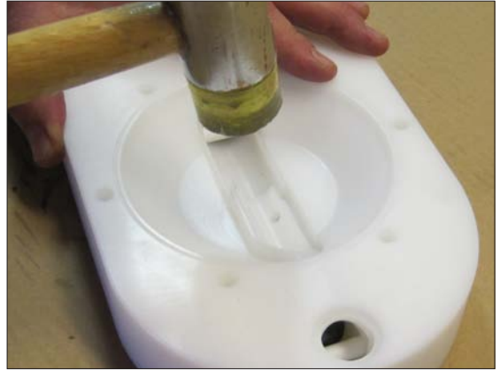
Fig 18. Make sure the seat and sleeve assembly is flat inside the housing.
