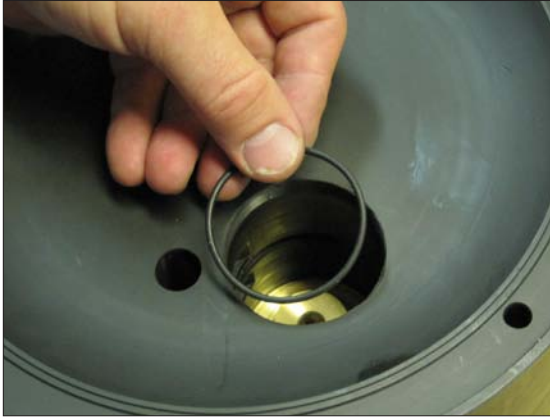
Fig 5. Place one of the o-rings (pos 30) on the endcap.
