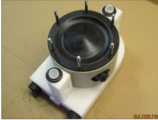
Fig 22. Put on the inlet and outlet connections (13), make sure all o-rings (18) are mounted.
