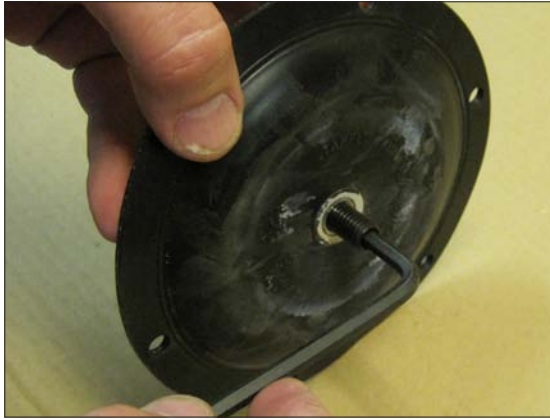
Fig 11. Mount the pin screw (part of the diaphragm shaft pos 16) securely in the diaphragm (15) by means of an allen key.
