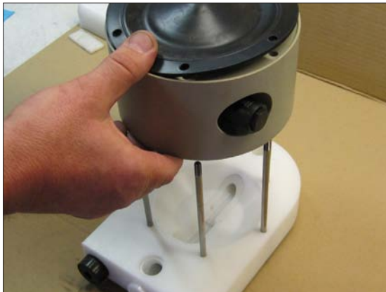
Fig 20. Make sure all pin screws (14) have one nut (37) and one washer (38) each. Nut should only be put on one or two threads. Put the pin screws through the housing and the stainless steel side plate and mount carefully the center block assembly.
