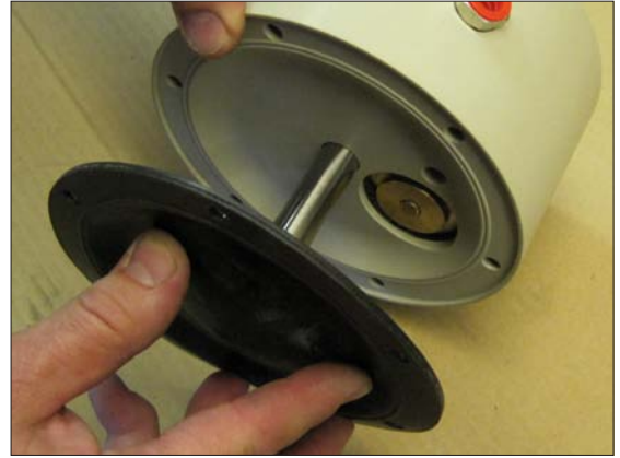
Fig 12. Mount the diaphragm shaft (16) on the diaphragm (15) and push the assembly carefully through the hole in the centerblock (12).
