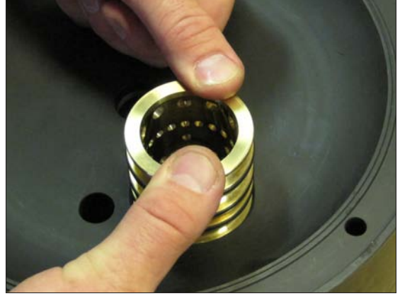
Fig 6. Make sure all four o-rings (pos 30) are mounted on the cylinder. Use a little water on the o-rings to easier slide the cylinder into the centerblock. Other lubricants should not be used.
