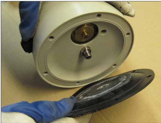
Fig 9. Press the diaphragms (15) to their neutral position (both have the same distance to the center block). Hold one of the diaphragms (15) and unscrew the other. Then pull out the remaining diaphragm (15) with the diaphragm shaft (16).
