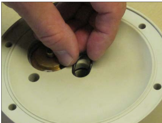
Fig 9. Insert the shaft seal o-rings (47) in the groove.
